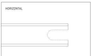
To reduce potential problems we recommend pushing the connection into the profile. It may be necessary to adapt (milling, boring) the aluminum profile for vertical connections or thick cables. Horizontal connections of cables in aluminium profiles may also be secured using adhesives where the connections / cable transitions are.
