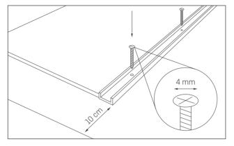
Cut aluminum profile (article no. 5901763) to custom-fit the respective installation and affix with 3 mm countersink screws.
