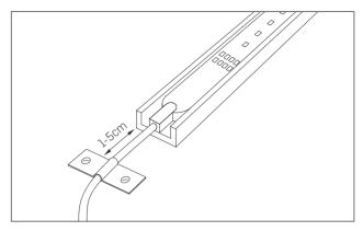
It is imperative that a strain relief be affixed  $1-5\,\mathrm{cm}$  from the connection to relieve any stress at the connection and attached wiring. This will be selected by the installer, depending on installation conditions and substrates. Please contact Döllken Lighting directly should you have queries or need recommendations.
