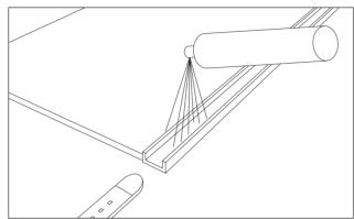
Uncoil the LED module and lay it out at the end of the installed aluminum profile. Use a little silicone spray at the start of the aluminium profile to facilitate insertion.
