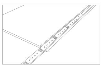
Insert the LED module into the profile end cap first, at a shallow angle and without kinking. Use more silicone spray, as needed.
