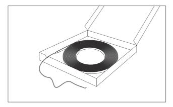
Take the LED module cable from the box, uncoil it and, if necessary, switch on for a while [max. 5 minutes] to raise the temperature of the product to  $18-30^{\circ}$ C for flawless installation.
