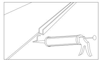
The aluminum profile may alternatively also be glued using suitable mounting adhesives (e.g. Sikaflex 221) and following the specific application notes.
