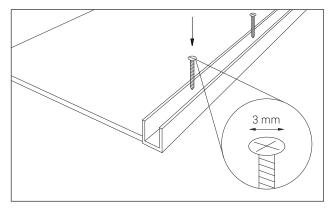
Cut aluminum profile (article no. 5902840) to custom-fit the respective installation and affix with 3 mm countersink screws.
