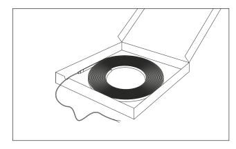
Take the LED module cable from the box, uncoil it and, if necessary, switch on for a while (max. 5 minutes) to raise the temperature of the product to 18 – 30°C for flawless installation.
