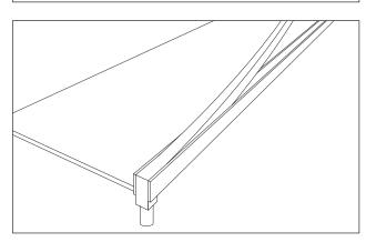
Gradually press the LED module into the aluminum profile at a shallow angle until it rests on the base. Never kink or use force to press the strip into the profile during installation since this may damage the sheath or conducting foil.
