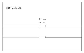
Ensure that expansion joints are included to absorb the expansion tolerances. The products will expand up to 2 mm per meter for each 10 Kelvin difference in temperature.
