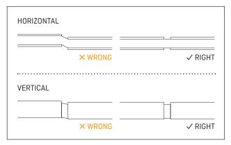
To avoid damaging the strip, the profiles must be horizontally and vertically aligned at the butt joints. They must also be adequately secured to prevent future movement.
