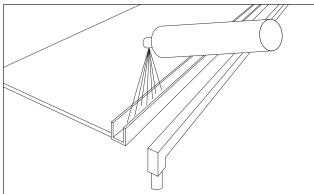
Uncoil the LED module and lay it out at the end of the installed aluminum profile.
