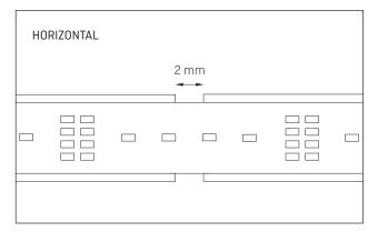
Ensure that expansion joints are included to absorb the expansion tolerances. The products will expand up to 2 mm per meter for each 10 Kelvin difference in temperature.
