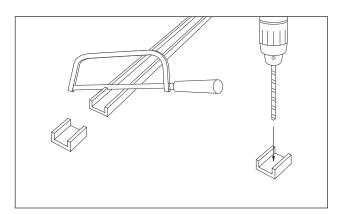
For an installation in various radiuses, the aluminum profiles can also be cut into small pieces and used as clips.
