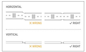
To avoid damaging the strip, the profiles must be horizontally and vertically aligned at the butt joints. They must also be adequately secured to prevent future movement.
