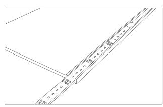
Insert the LED module into the profile end cap first, at a shallow angle and without kinking. Use more silicone spray, as needed.
