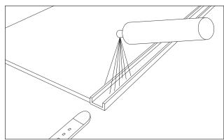
Uncoil the LED module and lay it out at the end of the installed aluminum profile. Use a little silicone spray at the start of the aluminium profile to facilitate insertion.
