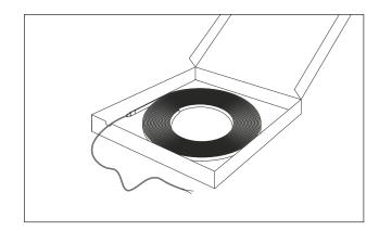
Take the LED module cable from the box, uncoil it and, if necessary, switch on for a while (max. 5 minutes) to raise the temperature of the product to 18 – 30°C for flawless installation.
