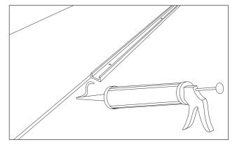
The aluminum profile may alternatively also be glued using suitable mounting adhesives (e.g. Sikaflex 221) and following the specific application notes.
