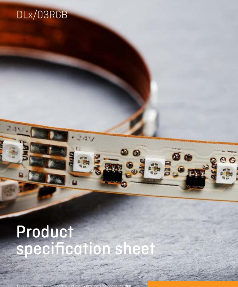
Our unprotected conductor film is primarily designed for indoor use, and its lack of sheathing enables it to demonstrate its full energy efficiency. The flexible LED strip can be installed with or without a self-adhesive strip and can be easily retrofitted to existing profiles.
