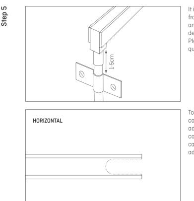
It is imperative that a strain relief be affixed 1 – 5 cm from the connection to relieve any stress at the connection and attached wiring. This will be selected by the installer, depending on installation conditions and substrates. Please contact Döllken Lighting directly should you have queries or need recommendations.
